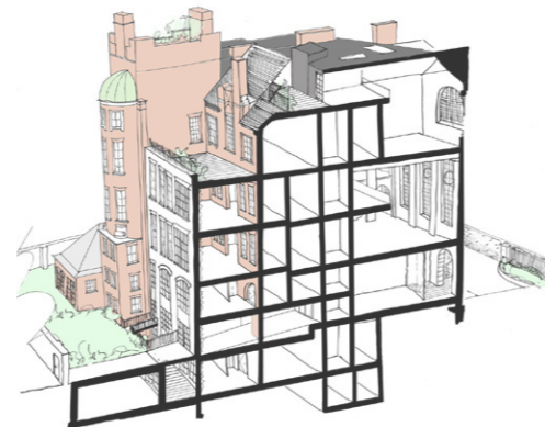
Axonometric section showing the double height gym above the main entrance at the front of the building with the private garden and terraces to the rear.
